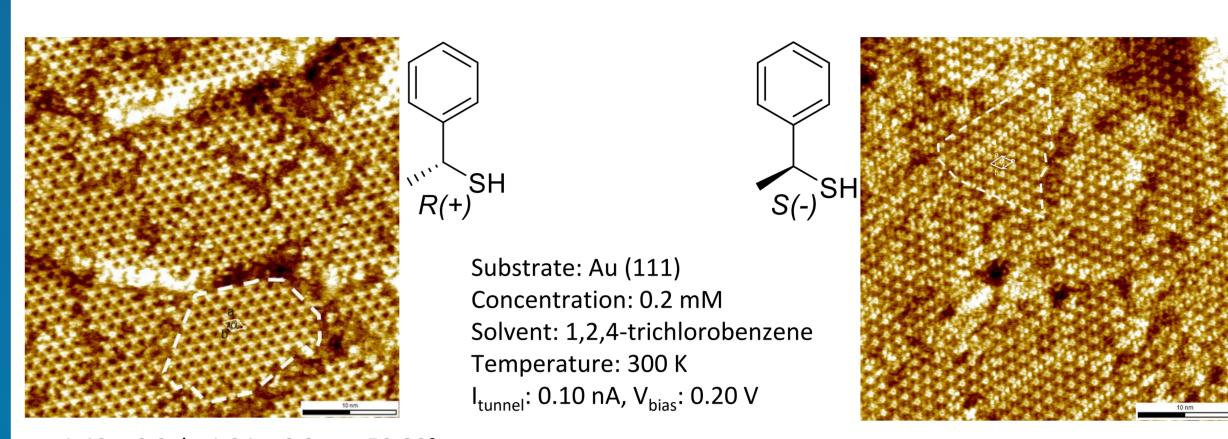
a:  $1.49 \pm 0.2$ , b:  $1.34 \pm 0.3$ ,  $\alpha$ : -59.80° a:  $1.42 \pm 0.4$ , b:  $1.35 \pm 0.3$ ,  $\alpha$ : -57.30° Inner area of the unit cell: 1.73 nm<sup>2</sup> Inner area of the unit cell: 1.78 nm<sup>2</sup>
